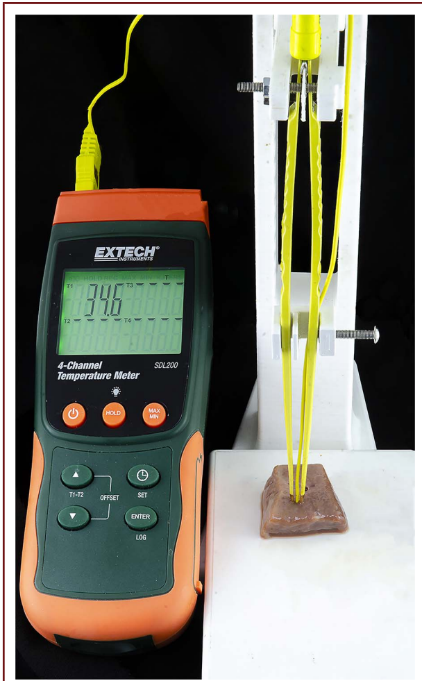
FIGURE 3. Thermocouple needle probes were placed into the tissue at the site of coagulation. A multichannel data logger captured temporal temperature changes up to a depth of 2 mm within the tissue.
